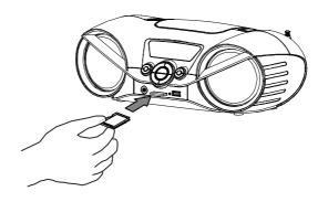
**Note**: The card can only be inserted one way. Push it in as far as it will go until it locks in place.
